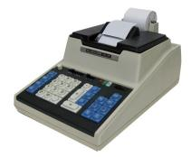
In the case of the Busicom 141-PF (also marketed as the NCR-18-36), the ROM contained the custom microprogramming to allow the MCS-4 chipset to operate as a calculator.
